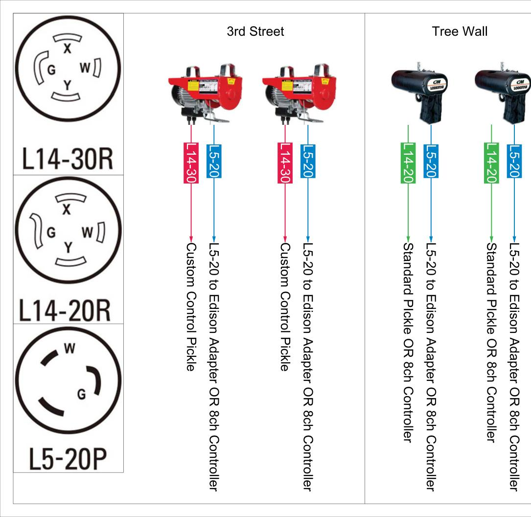
The 3rd Street and Tree Wall systems at Pearl are not compatible and must be operated independently. The L14 connections have been specifically configured with different connections to ensure this separation.
