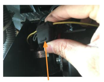
Once inside the box, the 15amp fuse is located inside this black housing. Replace if needed.
