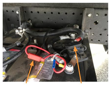
Under the battery cover on the left side of the truck you will find a 25amp fuse that can be replaced if needed.
