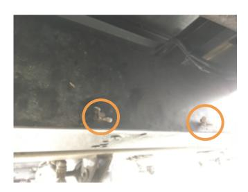
The last fuse is located under the truck just forward of the liftgate itself. The fuse can be accessed by removing the two wing nutes and removing the steel cover.
