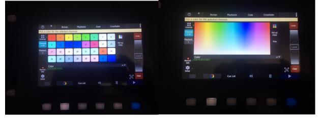
Recording a look onto a fader or "Playback Memory": After setting the desired look press <Record/Edit>, press the bump button of the fader the look should be assigned to. To playback stored "Memories" press <Playback 1> and make sure the Playback and Bumps faders are at 100%.
